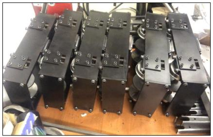
Six of the bogies now painted and assembly as most finished. There are another two to strip, paint and assemble. They can then be assembled along with the braking systems on to carriage frames.
