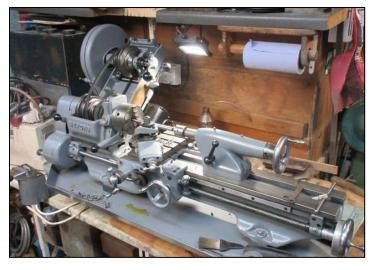
repair was the belt guard that had a crack to one corner I did try to MiG weld the aluminium casting but it really needs to be TiG welded alas I don't have a TiG welder?
