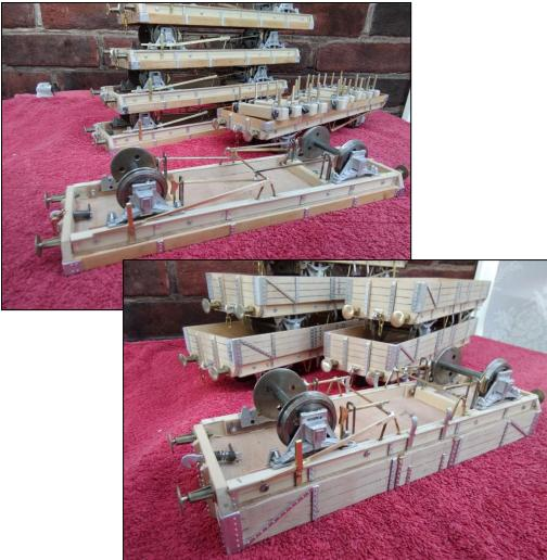
Metalwork is aluminium with a riveting tool used to add detail, purchased items being buffers, axleboxes and wheels only!
