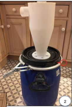
Now with the 3 components I started to assemble the revised cyclone: Drill a 67mm hole into the centre of the lid and 6 x 5 mm holes for the fixing roofing screws and nuts for attaching the cyclone to lid.
